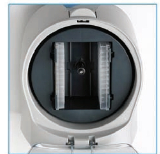
During centrifugation (Horizontal position)
